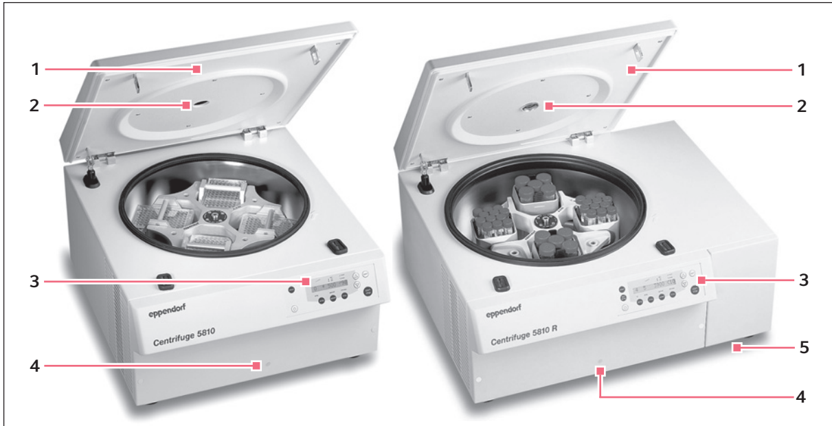
Fig. 12-1: Depiction of Centrifuge 5810 and 5810 R. The Centrifuges 5804 and 5804 R are similar in design.
